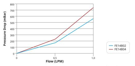
Tests performed in water @25°C
