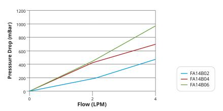
Tests performed in water @25°C
