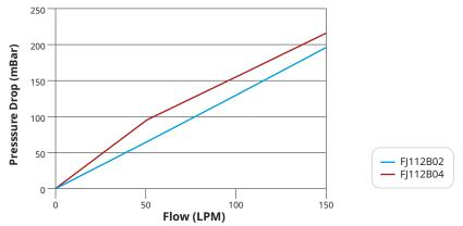
Tests performed in water @25°C
