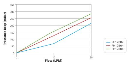
Tests performed in water @25°C
